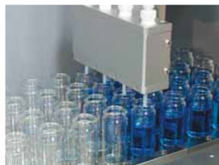
バイアルへの試薬・診断薬の高精度充填 Vials that are precisely filled with reagent or diagnostic medicine
